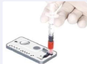
Step2: Add sample and slide the cap to seal the sample inlet.
